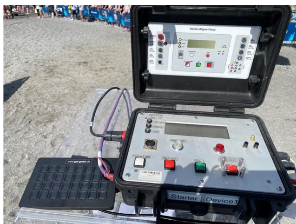
写真-14 Start Switch Box
